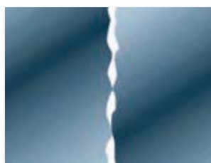
Typical interference fit has 30% metal-to-metal contact.
